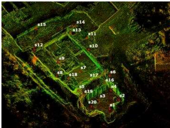
Figure 7. Topographical network for the laser scanning stations.
