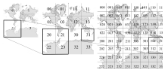
Figure 8. Representation of quadkeys used to identify images in tile server.
