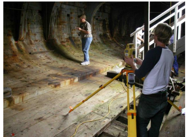
Figure 1. Placing reflective targets on the floating vessel Wawona , with a total station and a TDS Recon unit in the foreground. Photograph courtesy of Nat Howe and Northwest Seaport.
