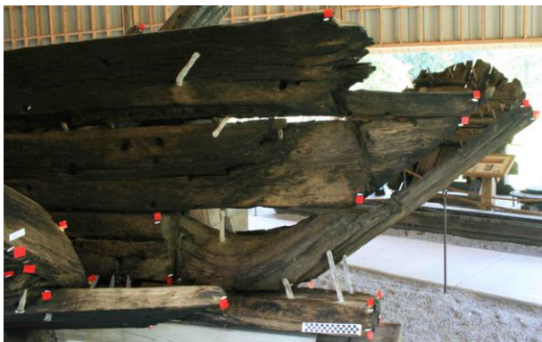
Figure 2. One inch square targets cut from reflective tape on the bow of the CSS Neuse .
