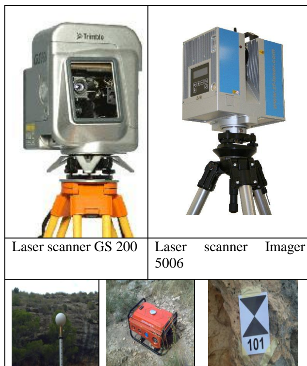
Figure 5. Equipment and photographs of the spheres, generator and targets used.
