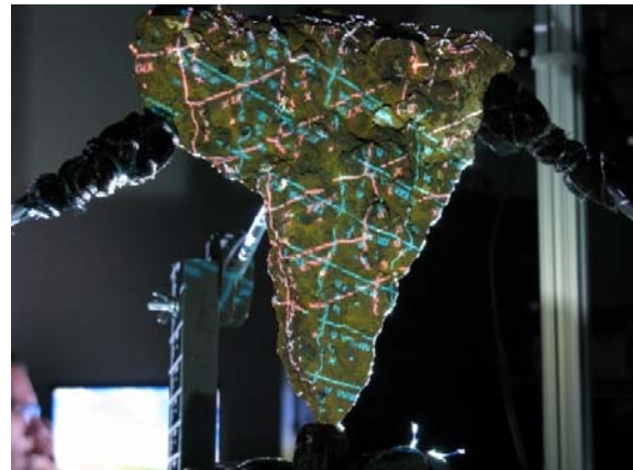
Figure 4: Fiducial patterns remained fixed in on surface during rotation of artifact.
