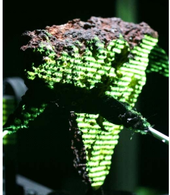
Figure 7: A single PMP pattern projection.
