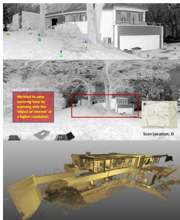
Figure 4. High resolution scan of the 'object of interest' after low resolution over all scan (top). An example of post-processing (bottom).
