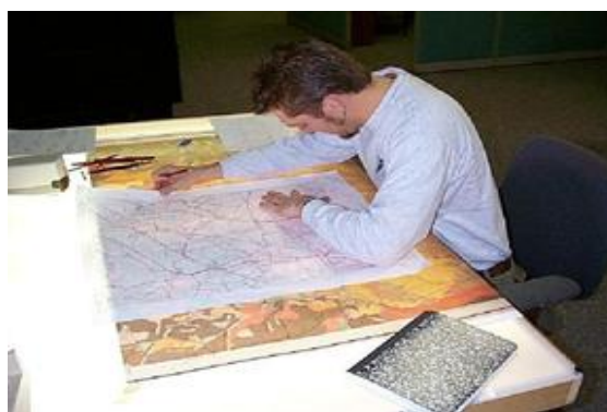
Figure 4. Manually transferring features from enlarged color map onto mylar
