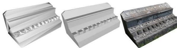
Figure 6. A model of a find showing wrong normals orientation.
