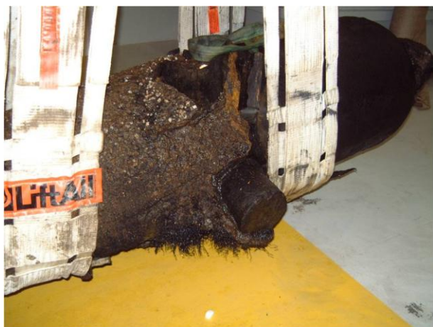
Figure 2. A CSS Alabama Cannon partly de-concreted. CCC 2009.
