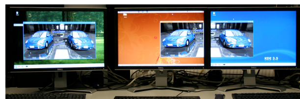
Figure 8. Real-time ray tracing simultaneously displayed on three presentation hosts, all of which are fully interactive and synchronized. The image is rendered on a cluster of six machines, and displayed in a single window on one computer (left) and a display-wall via two split video streams on two additional machines (right).
