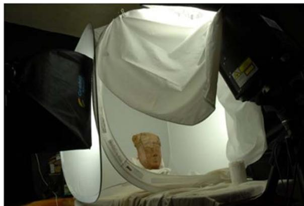
**Figure 7.** Professional light tent with scanner array.
