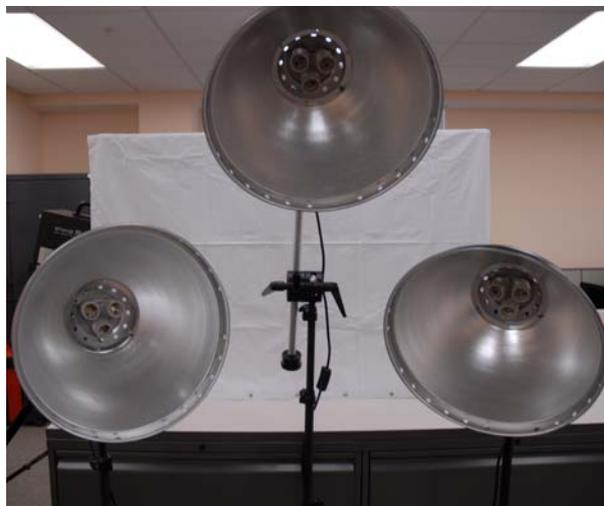
**Figure 8.** Aluminium 17-inch reflectors.
