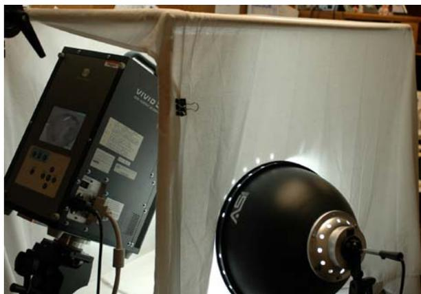
**Figure 6.** Light tent with scanner array.
